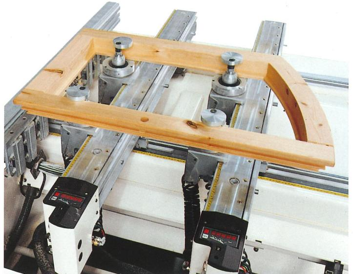
TVN worktable enables fast machining changeover:
