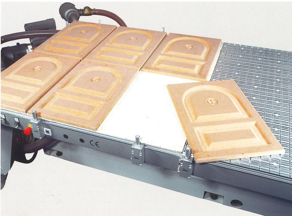
Ideal for vacuum hold-down clamping because it ensures high vacuum capacity, constant in each worktable area
