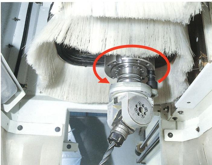
**Vector rotary axis** for routing, sawing and drilling on tilted axes using angle drive heads
