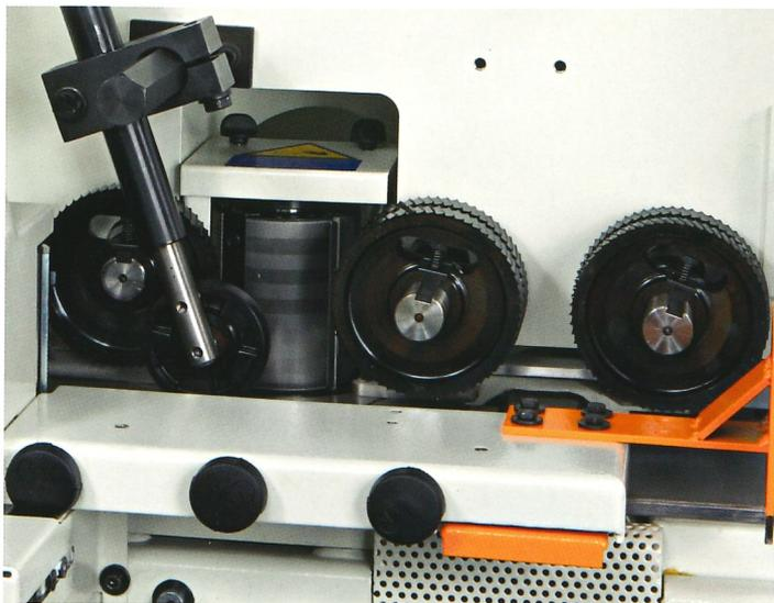
**Quick-release feed unit positioned before the surfacer (option):**
