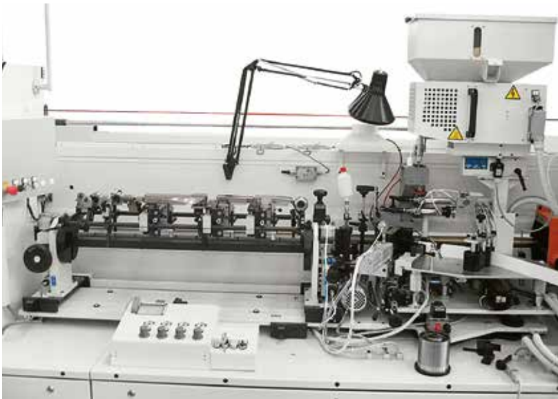
Gluing unit for thin/soft edges doors processing.
