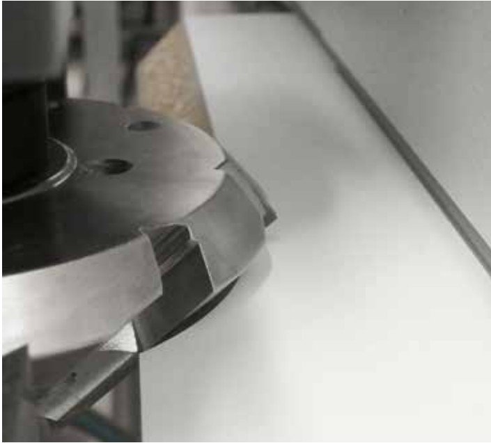
HSK tools for a quick and precise setup for different profiles.
