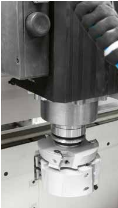
MX80 HSK SOFT profiling unit with quick tool change.
