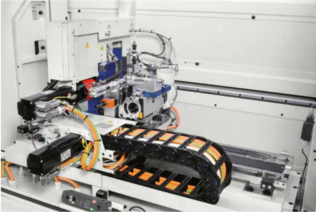
Servo-driven rounding unit, Round J-side, designed for the complete finishing of J and C type profiles.
