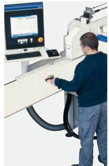
SIMPLE ACTS, ADVANCED TECHNOLOGY Automatic program set up by Bar Code device
