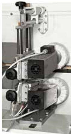
Rotating brush device for the brightening and the final cleaning of the applied edge.
