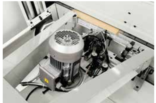
Sanding unit for profiled panels.
