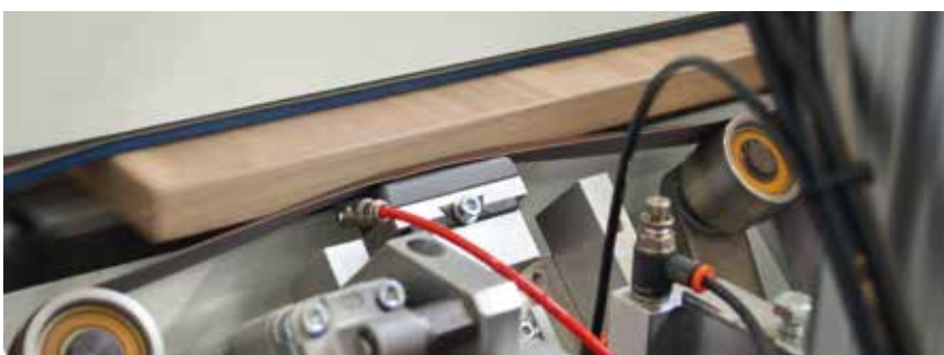
Sanding unit for chamfers/radii.
