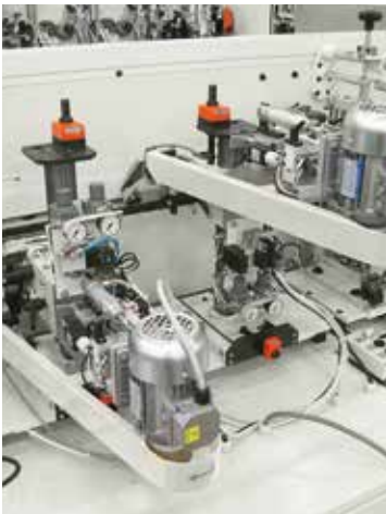
Sanding unit for chamfers/radii.
