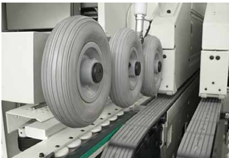
Approach system to the entry guide for machines in the version for only longitudinal pass machining.
