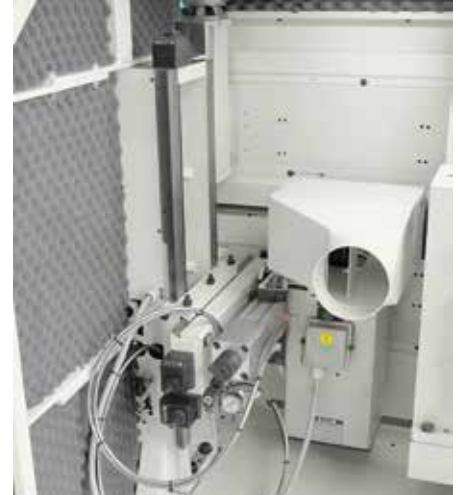
Milling unit. Ideal for grooves.
