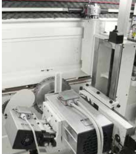
Hogging + scoring unit. Ideal for veneer panels.
