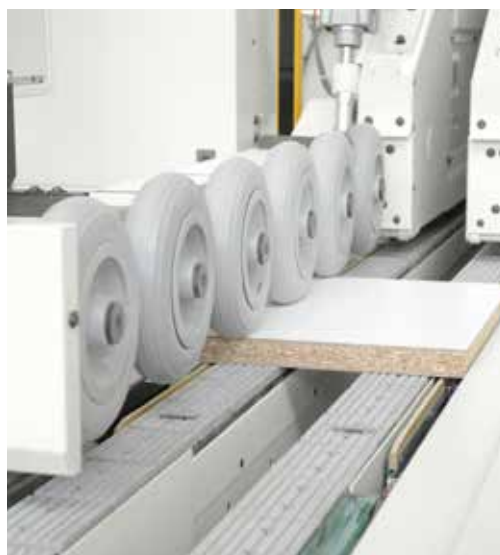
Approach system to the entry guide for machines in the version for longitudinal + transversal pass machining.
