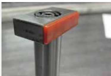
Double dog system for the precise and constant transport of the panel along the entire machine for the transversal processing. To ensure the maximum possible production with each panel size, the dog pitch can be chosen among: 900 mm, 500 mm, 400 mm, 300 mm. Dogs are adjusted automatically in height.
