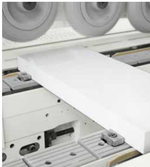
Double dog system for the precise and constant transport of the panel along the entire machine for the transversal processing. To ensure the maximum possible production with each panel size, the dog pitch can be chosen among: 900 mm, 500 mm, 400 mm, 300 mm. Dogs are adjusted automatically in height.
