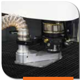
Suction inlet on the cutting head
