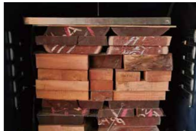
The pressure plate is made of stainless steel 304
