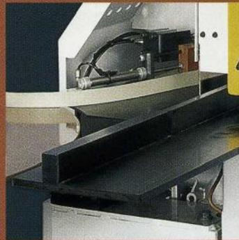
◀ Large infeed guide, to ensure safe loading of panels of all sizes.
