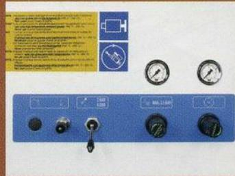
◀ Quick selection switch for pneumatic pressure of the shearing device: thin edge - 2-3 mm thick edge. Adjustments and controls on independent devices.
