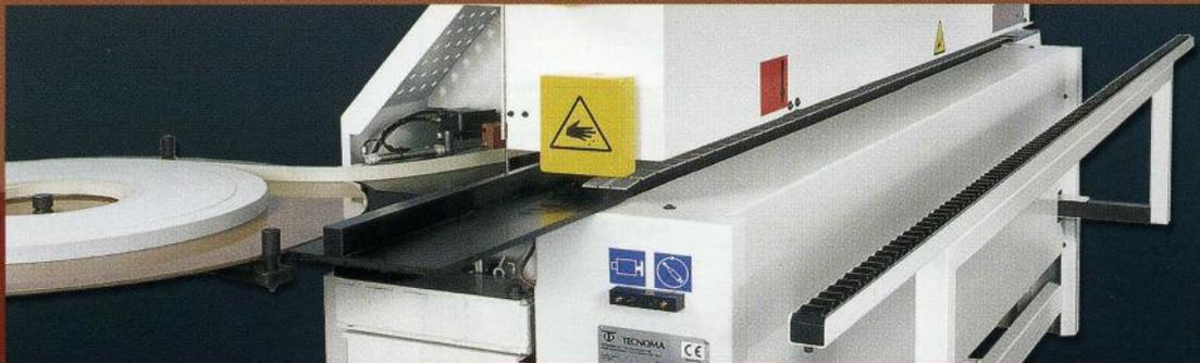
◀ Adjustable rollers support for large panels, running the entire length of the machine.
