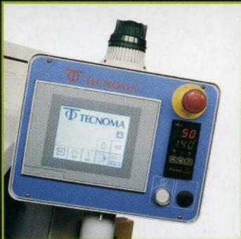
◀ Programmable logic control with PLC with operator interface with monitor "touch screen".
