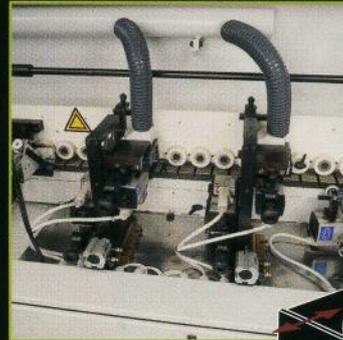
◀ Quick pneumatic release of working units from the control panel.
