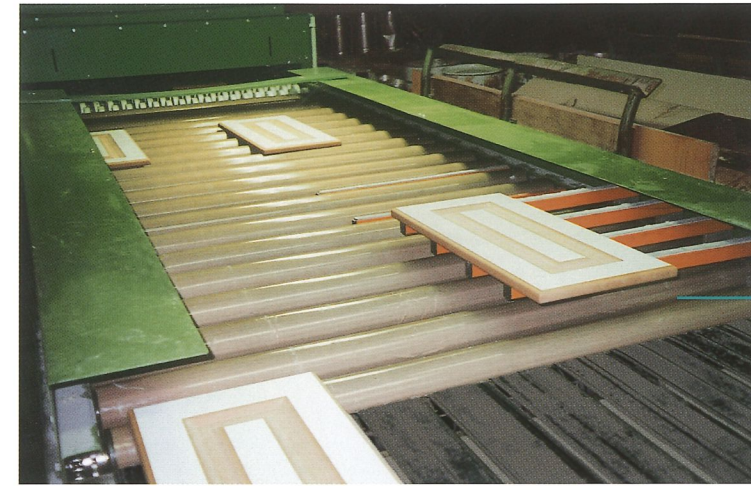
Roller conveyor with workpiece transfer station, from single to double track
