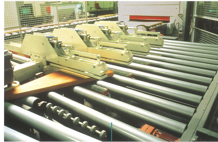
Turning station for processing the surface of workpieces on both sides
