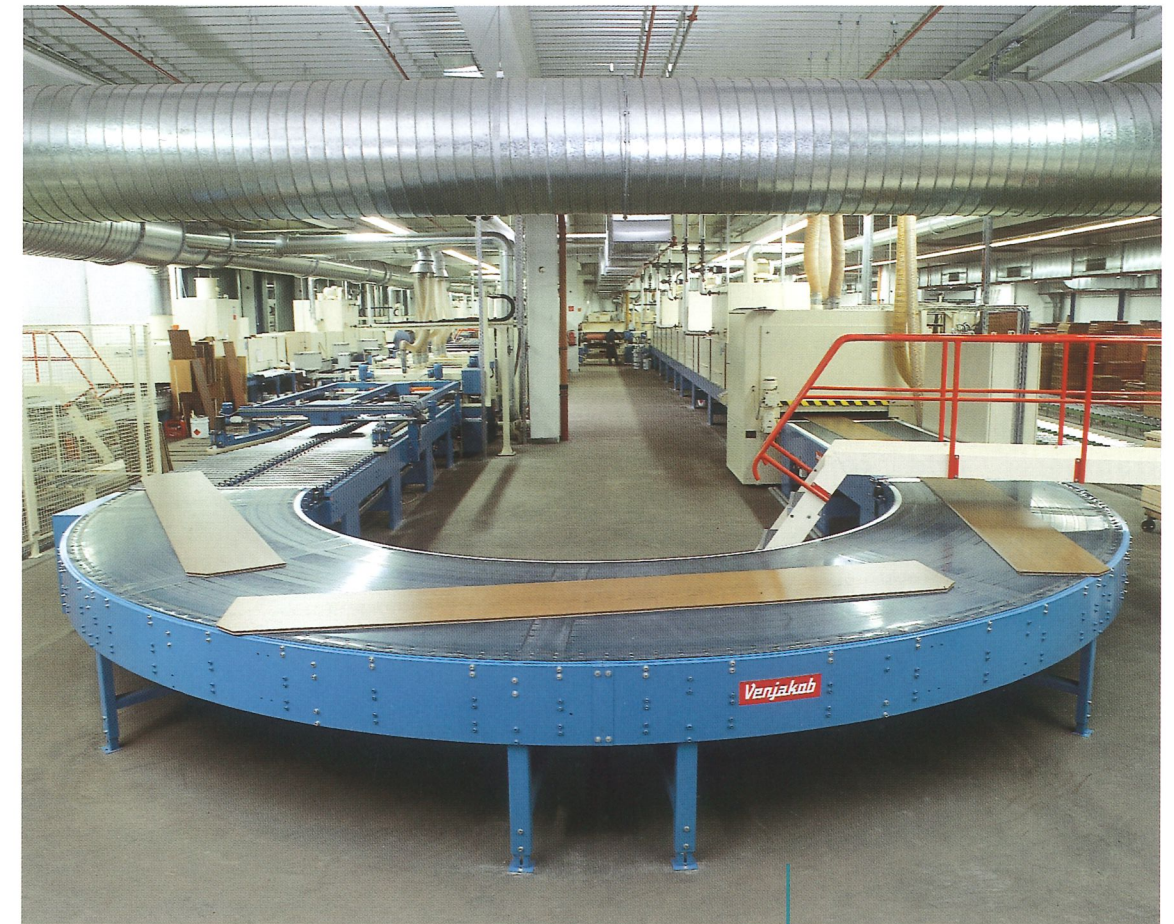
Returning parts by means of a 180° conveyor belt curve
