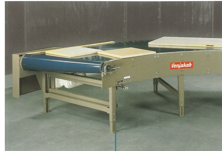
Partial view: workpieces can project in the inner radius
