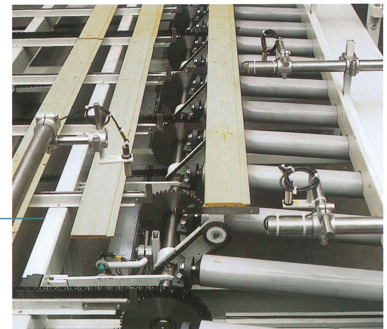
Workpiece separation by means of eccentric-operated cams, from crosswise transportation to lengthwise
