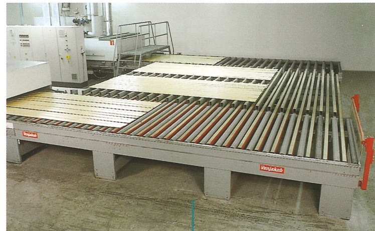
Grid-angle transfer 180°, used as a workpiece return device
