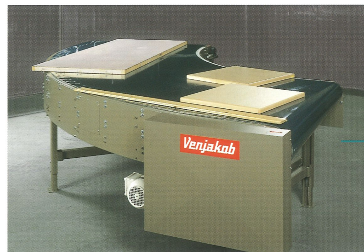
Partial view: workpieces can project over the outer radius
