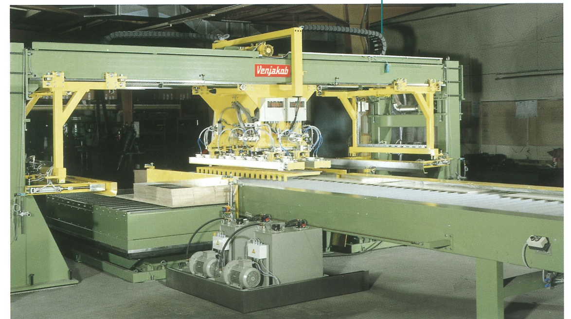
Double-sided, high-performance automatic stacking machine with workpiece alignment
