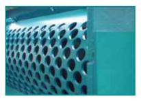
The size of the chips is determined by the inserted screen perforations. The design of the screen perforation size is dependent on the subsequent use of the chips.
