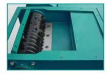
Via the standard installed pusher the material is pressed against the rotor shaft. The stripper band prevents thin materials from getting stuck between the pusher and the machine board.
