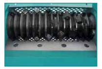
The insertion of concave cutting tools (quadruple rotation) makes high chipping power possible even with hard materials. Eight times rotating KARO cutting tools guarantee a long knife life.
