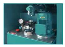
The hydraulic aggregate is fully integrated into the machine body. Hydraulic cylinder is gimballed stored thus ensuring a long life span.
