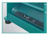
Foreign metal objects such as nails, screws or metal clips can be sorted out after the shredding by means of an optional permanent magnet.
