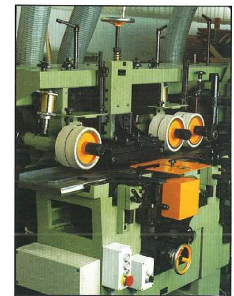
▲ 44 In planing and moulding mills thin and wide material is machined very often. For this purpose we use a special top guide, i.e. opposite to the bottom Rotaplan spindle.
