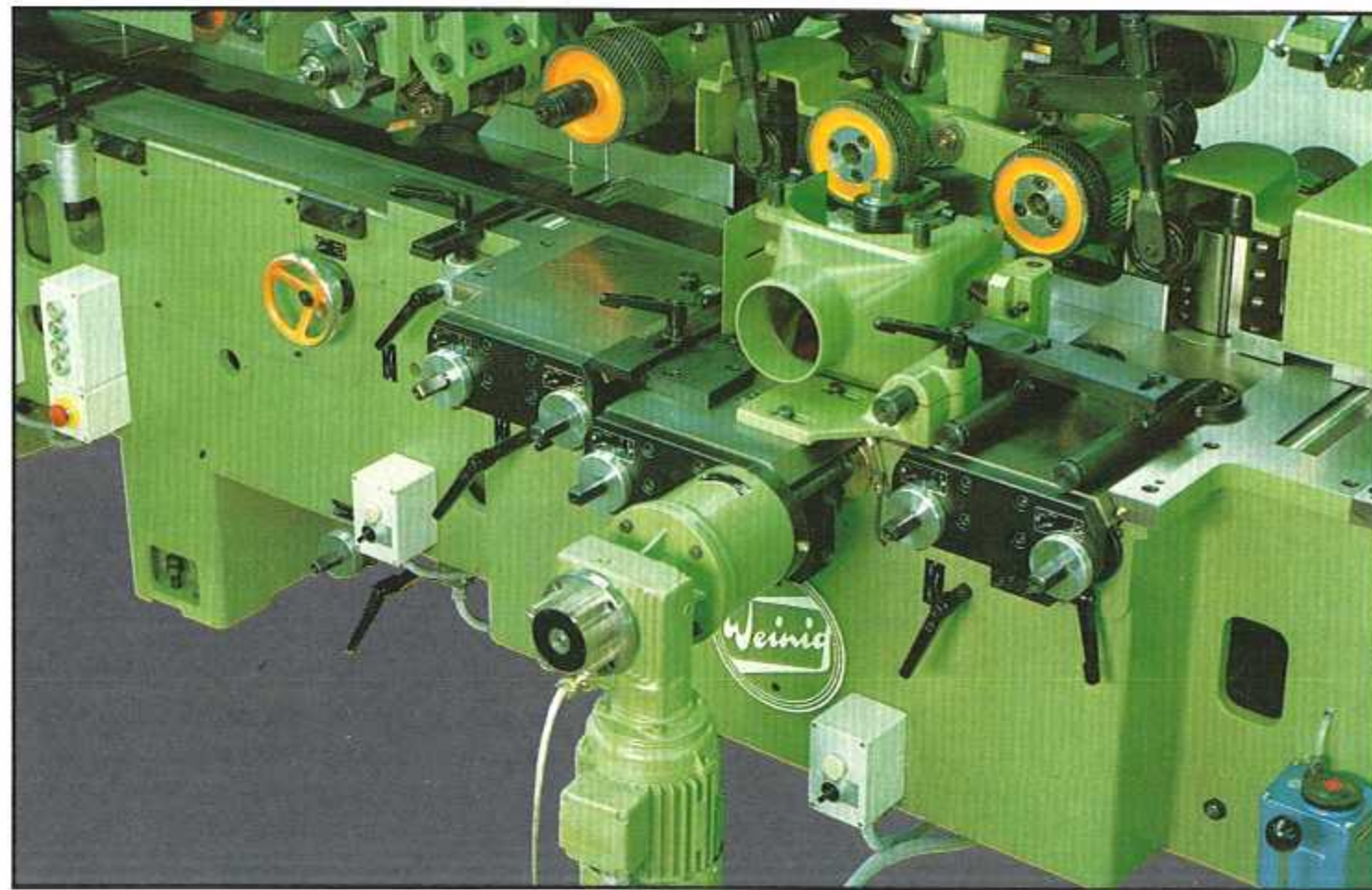
◀ 82 Precision workpiece dimension is also required when sawing. The use of a special table plate for wood inserts produces a closed table surface so that the workpieces can be split with high accuracy.
