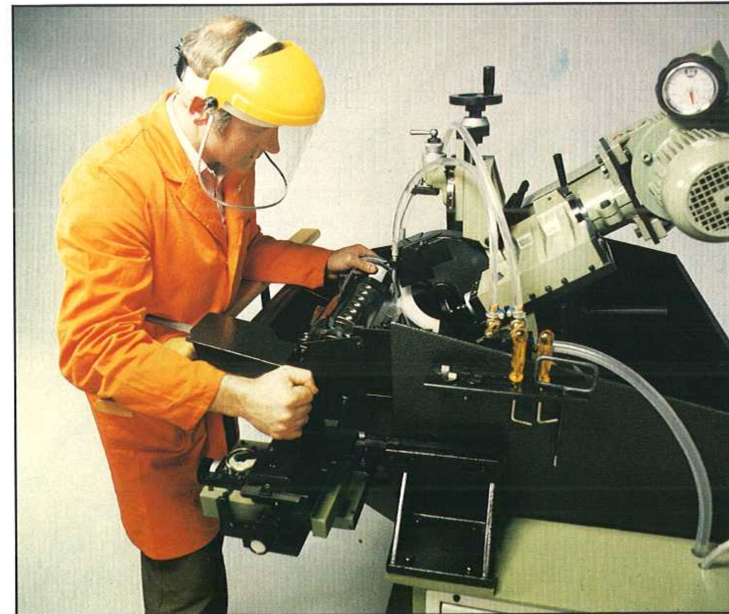
▲ 89 The Rondamat 929 – an inexpensive profile grinder. The machine which makes small and medium sized shops independent from tooling suppliers.
