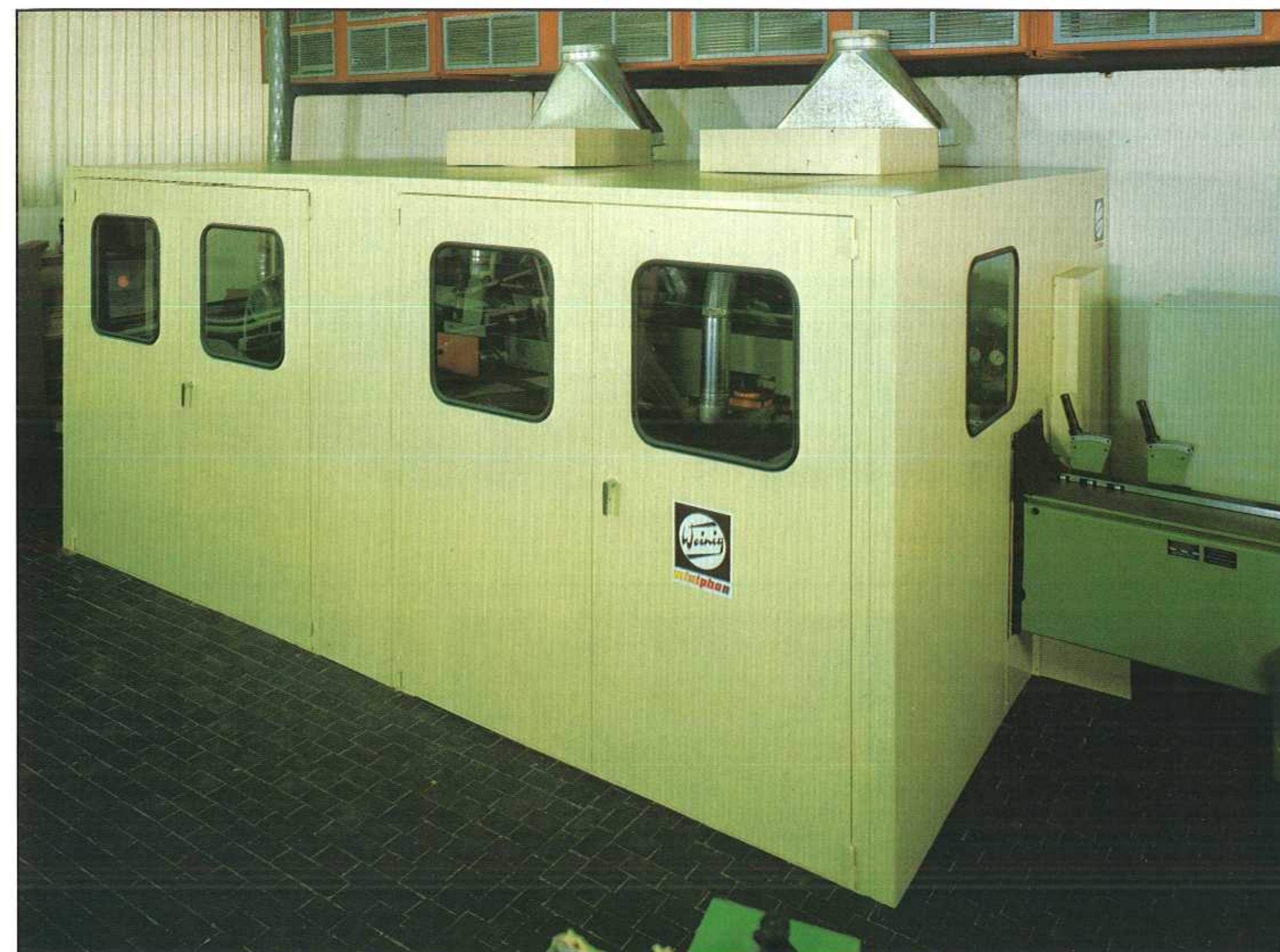
▲ 105 The Miniphon 100 enclosure is the lowest priced and most popular version in our range. Tailor-made from standard elements. Installation by you according to supplied instructions. Can be extended for modified or new machines. Simple machine operation through large doors. Easy accessibility for maintenance and repair work.
