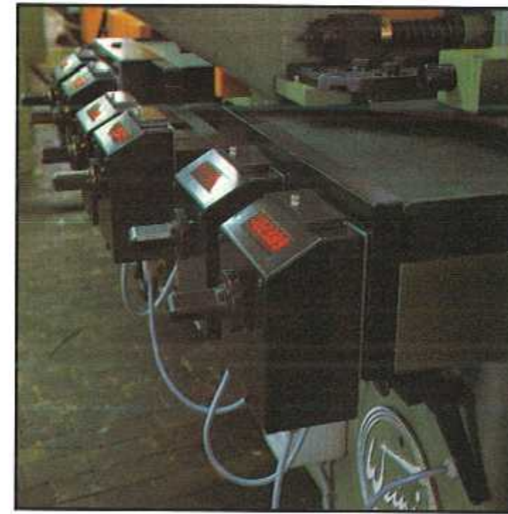
▲ 75 The EMA calculators with electronic display systems are located directly on the setting spindle.
