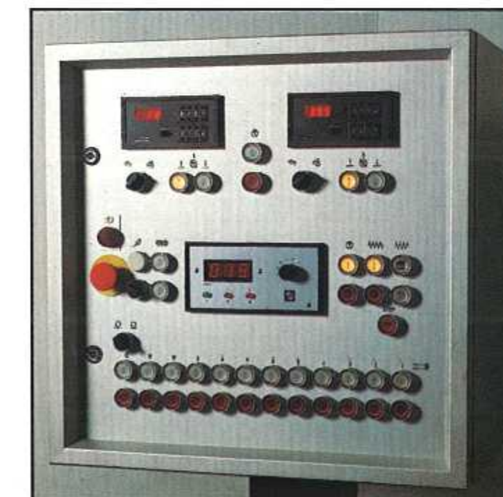
◀ 24 On the moulder control panel all the controls for the jump spindle are integrated.
