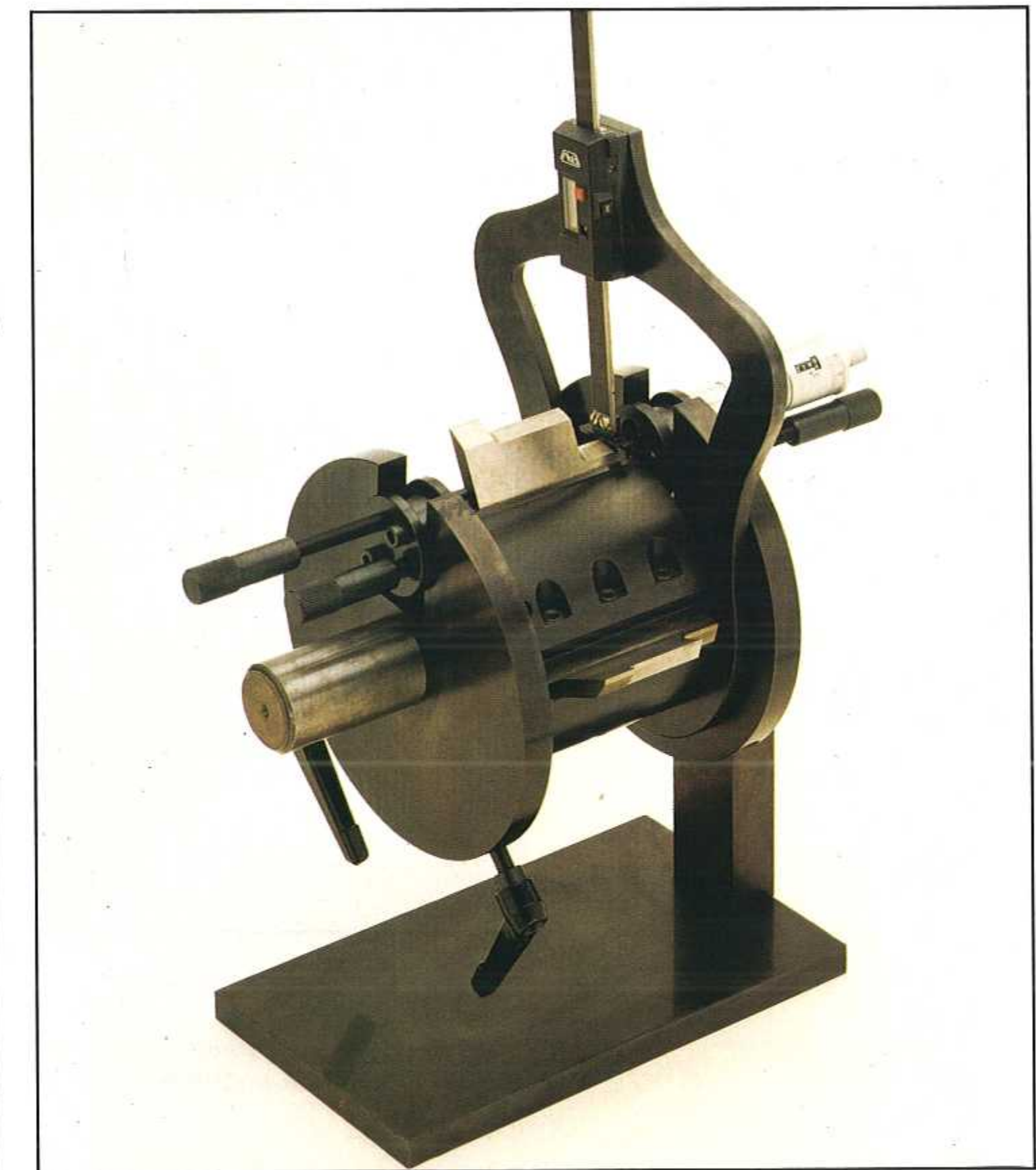
◀ 102 The standard setting stand for planer heads – a low priced, reliable and accurate instrument.
