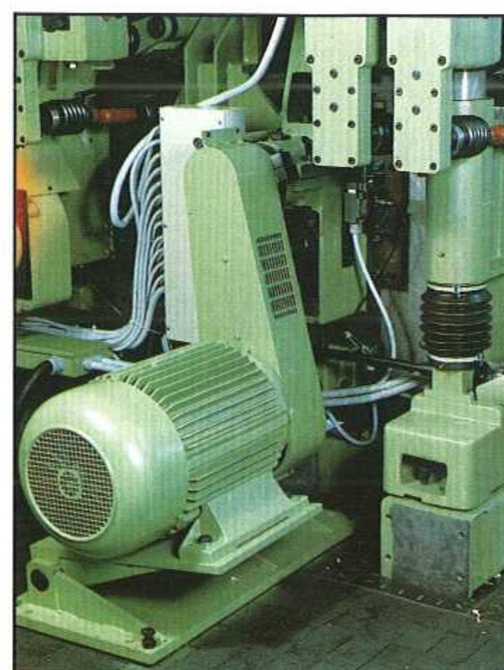
► 83 Here is a 37.5 kw (50 hp) motor to drive a splitting spindle. This means that sawing is also possible at high feed speeds and with several saw blades and large workpiece dimensions.
