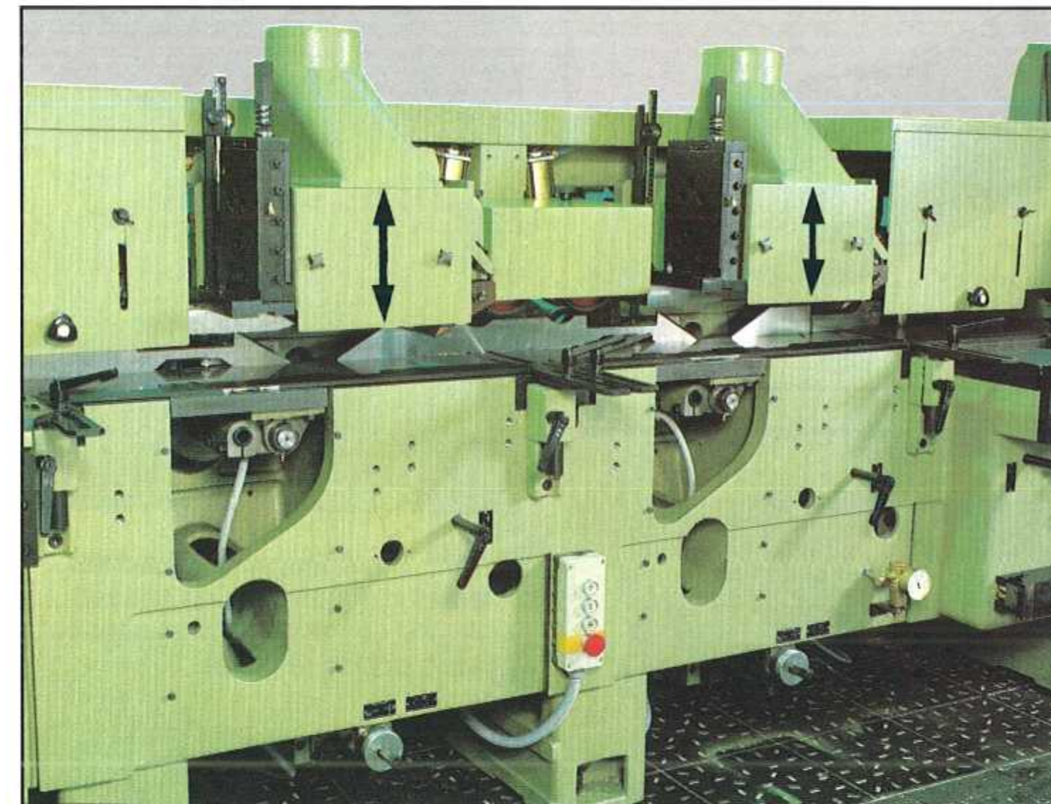
◀ 23 Jumping, i.e. non-continuous profiling, can be performed fully automatically on the moulder for various kinds of productions.
