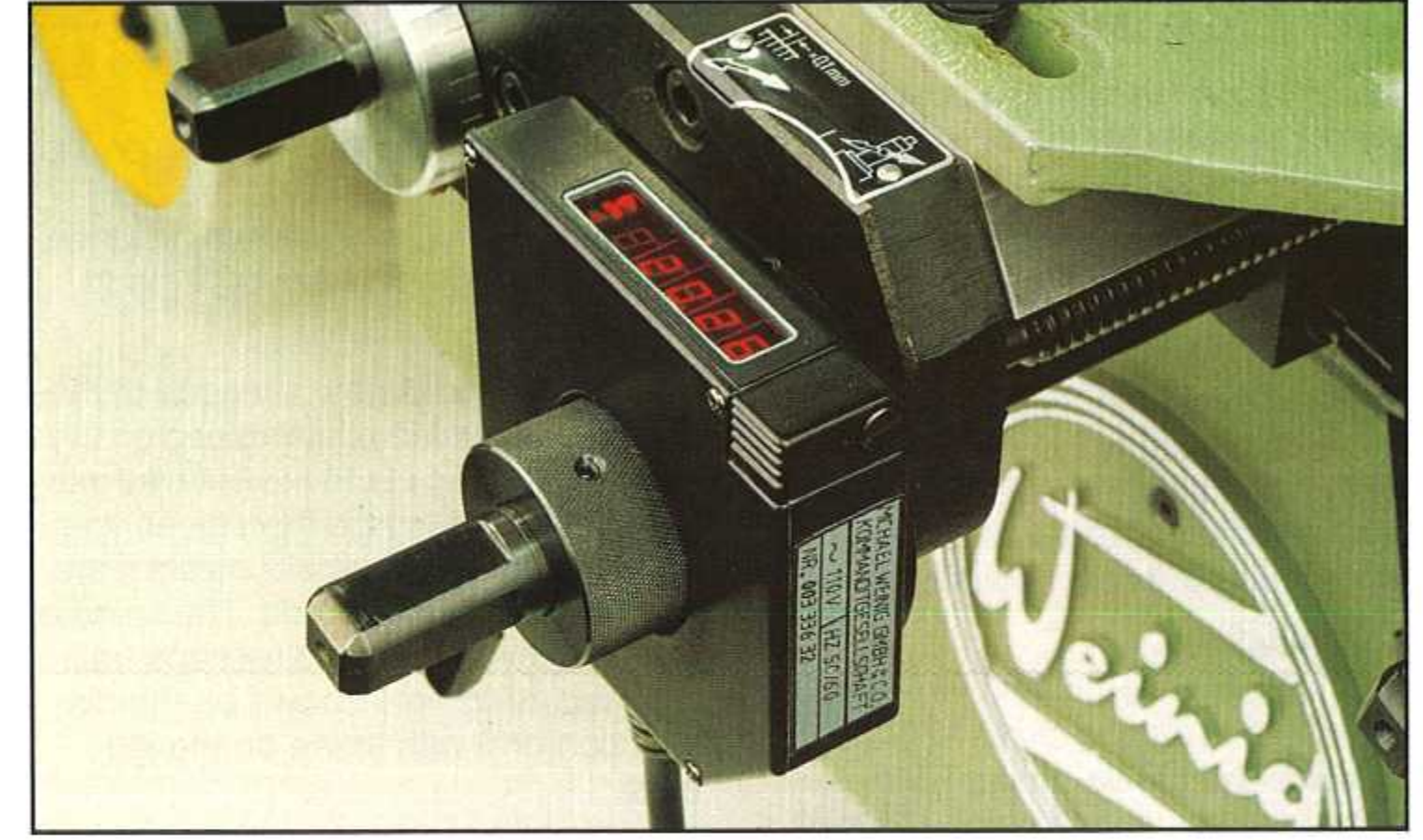
▲ 71 The electronic digital display is even more accurate and quicker.
