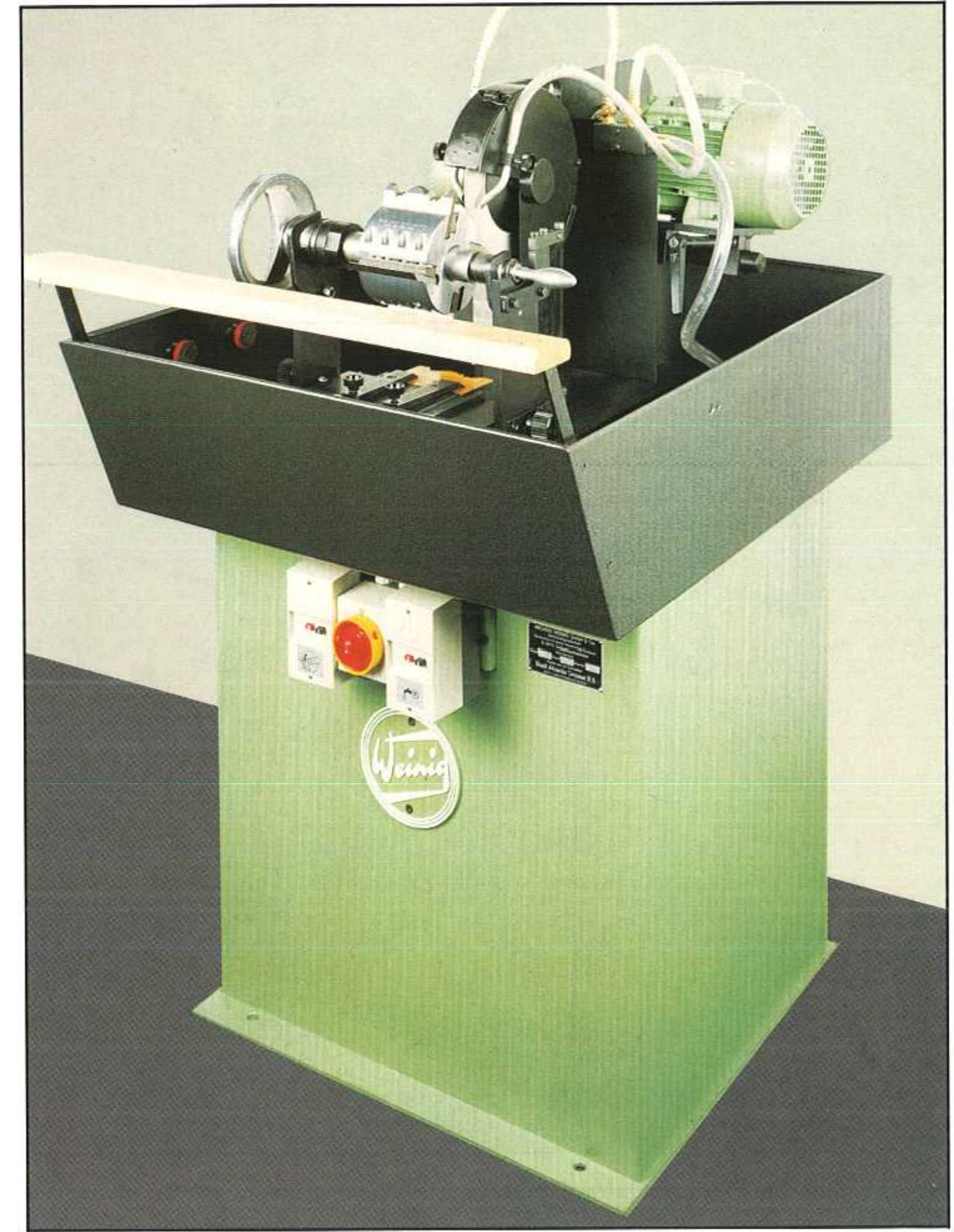
▲ 89 The Rondamat 929 – an inexpensive profile grinder. The machine which makes small and medium sized shops independent from tooling suppliers.
