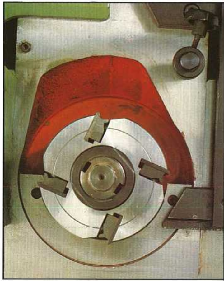
▲ 66 Insert sections on vertical spindles provide a closed table surface which is particularly important when producing extremely narrow profiles.
