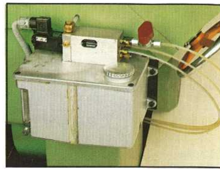
▲ 61 High speed machines are usually equipped with an automatic lubricant pump . The pumping intervals are determined by an adjustable time relay in the switch cabinet.
