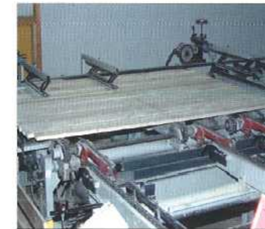
Feeding the moulder. Reasonably priced lateral chain feeders for feeds up to 80 m/min are available. Higher feed speeds upon demand. Cross-conveyors with or without automatic separating systems are used for higher feed speeds on heavier workpieces, and can be combined with various high-speed accelerators.
