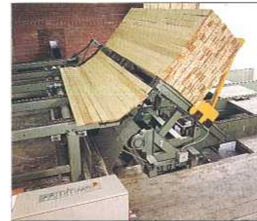
Automating the unstacking process The lifting table facilitates feeding the moulder. Tilt unstacking is recommended for speeds of more than 80 m/min, moving layer after layer in a favourable position to the operator. A fully automatic unstacking system is also offered pushing off the layers in lengthwise direction without any manual intervention.
