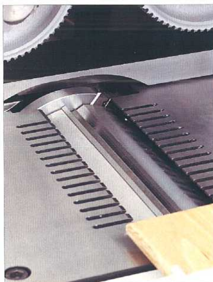
Straightening spindle with rebate cutter and slotted table plates The rebate cutter provides a reference cut for increased straightness and edge-gluing accuracy. The special table plate design helps reduce noise.
