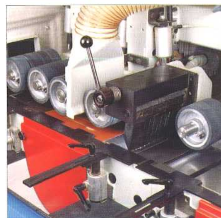
Anti-kickback device A "must" for sawing work and the production of multiple profiles. It prevents kickback and possible injuries to the operator.
