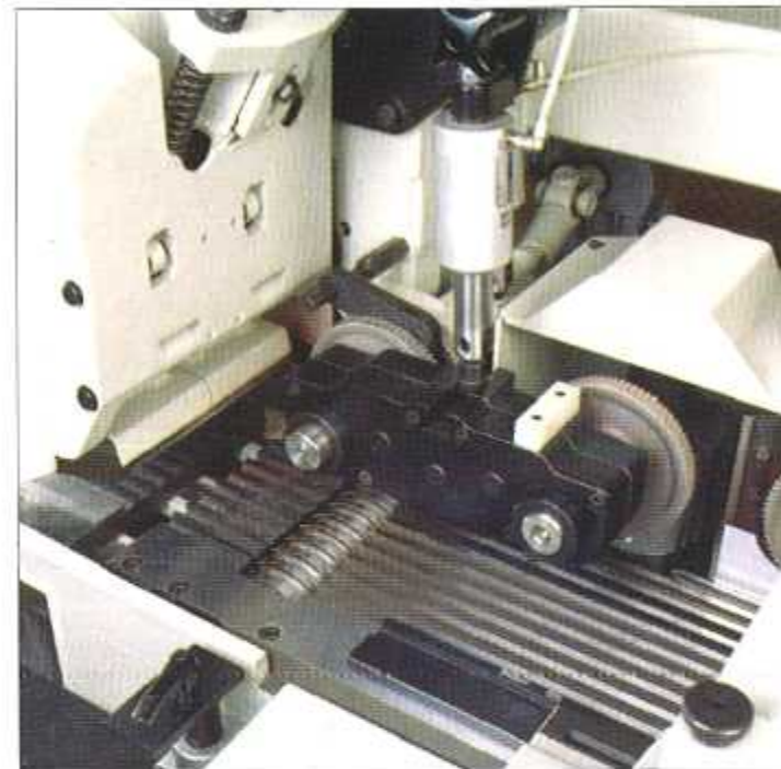
Protection against tear-up Useful when processing very short workpieces as it prevents the feed roller in front of the top spindle from pulling the work-piece upwards.
