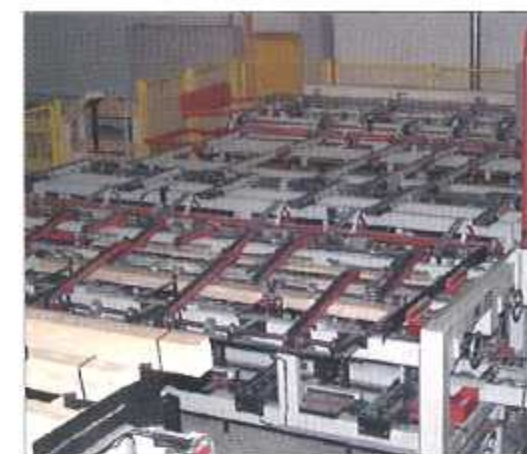
Automating the bundling process When a marketable presentation is demanded: Semi-automatic as well as fully-automatic bundling systems are offered, for bundles of slats and for packages of tongue-and-groove goods.
