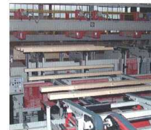
Automating the stacking process A semi- or fully-automatic stacker can be selected depending on the output of the planer or moulder. The major stack which may be made of small packages or bundles is produced fully automatically. A special stacker is available for the mini-packs that are always in demand in the market.
