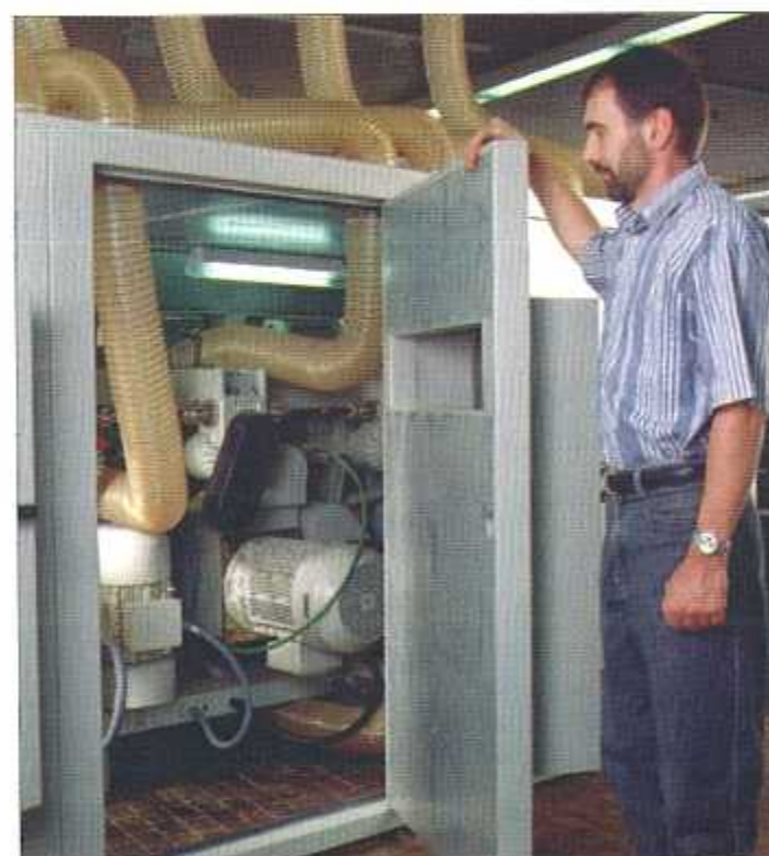
Increased sound insulation Even though the standard enclosure on our moulders comply with the CE standard, this increased sound insulation reduces the noise by up to another 18 dBa. No reduction in machine accessibility.
