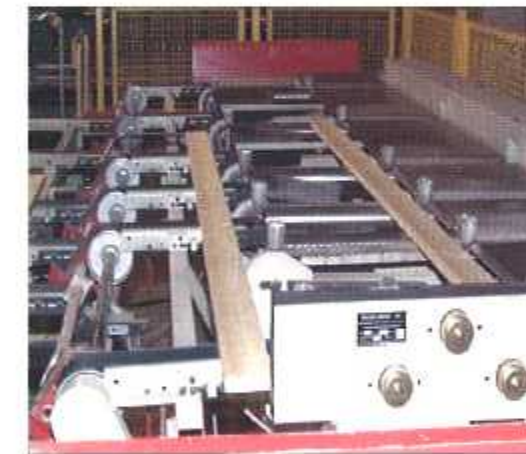
Automating the cross transfer process A variety of products demands a variety of solutions - which we can offer. The functions of the cross transfer can be assumed by arms, cylinders, belts or chain feeders, or even flippers and slideway fences. Directly connected do the cross transfer is the turning and lowering of workpieces. Sliding or dropping of parts can be integrated as well.
