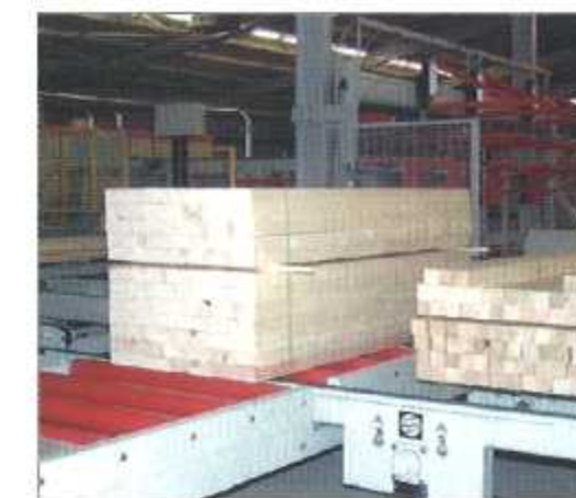
Material transport. Various devices are available for the lengthwise and cross transport of raw and finished products. Roller paths or conveyors transport in lengthwise direction; their design depends on the weight of the workpieces. The cross conveyors were given extra attention keeping in mind that they have to move finished individual parts or packages without causing any damage to them.
