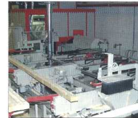
Automating the processes of end trimming and cutting to length Cut-off saws are available as one-sided or multiple saws. They independently carry out both final end cuts or produce multiple short fixed lengths ... or according to specified modular dimensions.
