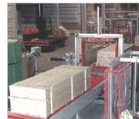
Automating the bundling and packaging process. The lengthwise bundler manages up to three packages per minute. Cross bundlers have a higher throughput. Small bundles are tied with cord or plastic strips. Shrink wrapping is recommended for high output and stretch foil wrapping for lower capacity.
