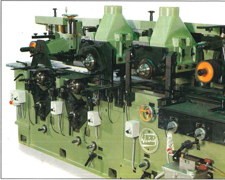
By extending the number of spindles even complicated profiles can be produced.
