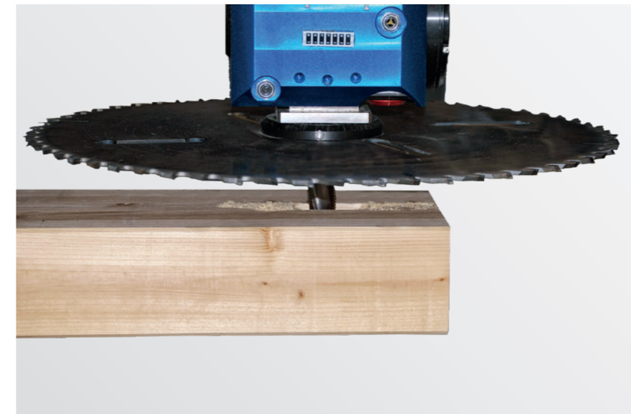
Saw blade with integrated routing unit
