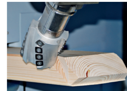
Producing a tenon joint
