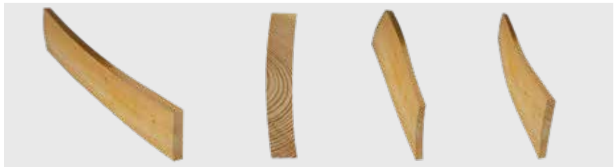
Blocks with longitudinal/latitudinal deformation, cupped or warped
