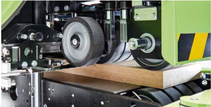
Driven feed rollers at top and bottom
