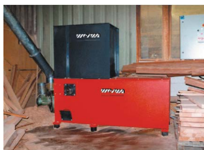
WL 4 S series shredder, for shredding of wood
