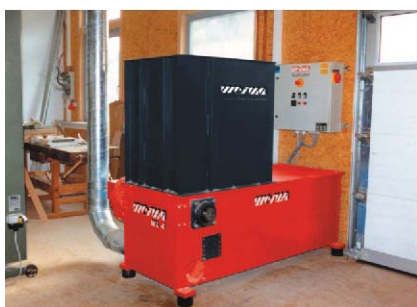
WL 4 series shredder, connected to an extraction system
