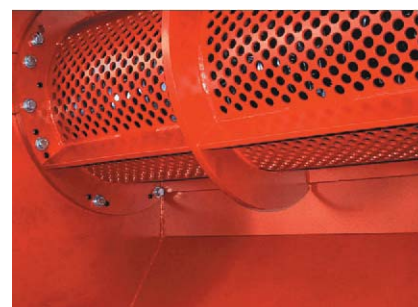
The screen size perforation determines the chip size
