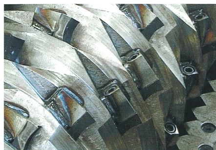
V-rotor with two knife rows
