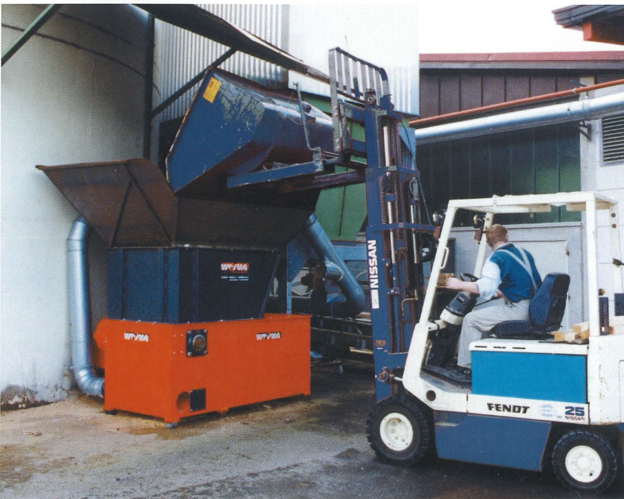
WL 6 S series shredder, material loading by fork-lift truck with tripper
