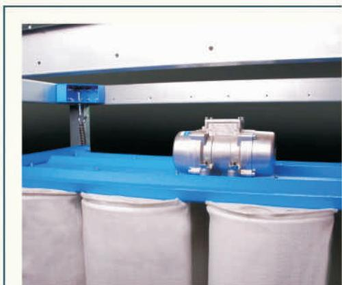
Filter hose regeneration via vibration motor
