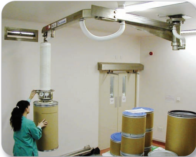
Knuckle Jib - Ceiling Mounted
