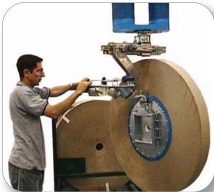
Vacuum Grip - Pneumatic Push Button Rotation
