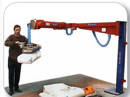
Low Headroom - Horizontal Tube
