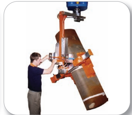
Pneumatic Grip & Rotate
