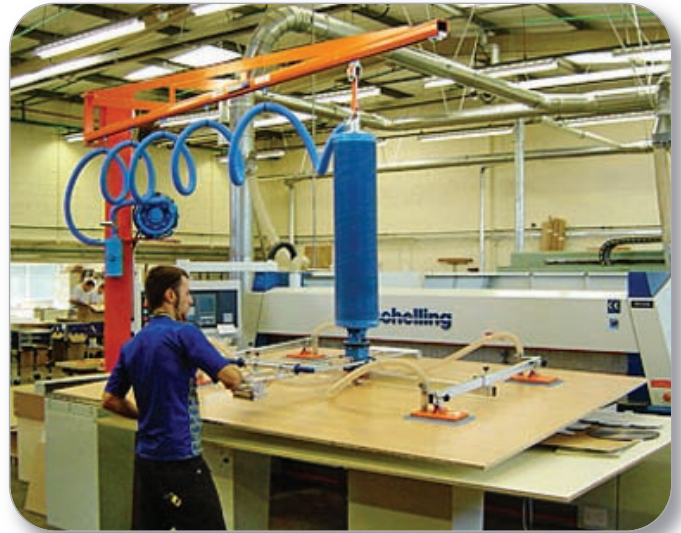
Panel Doors & Large Panels Suction Foot
