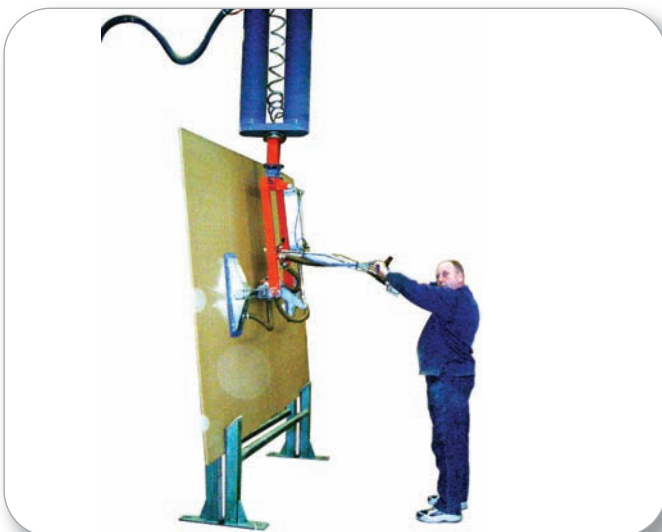
90° Powered Turner - Large Panels
