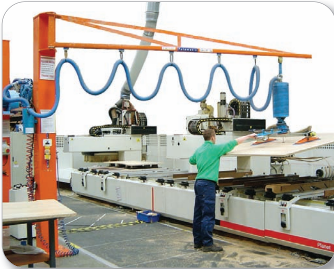
Door Blanks & Small Panel Suction Foot
