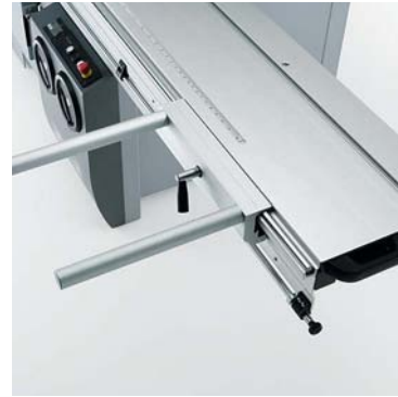
STEG: second support on the sliding table (width 400 mm).
