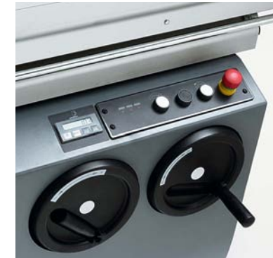
Manual rise/fall and tilt adjustment of the saw blade.
