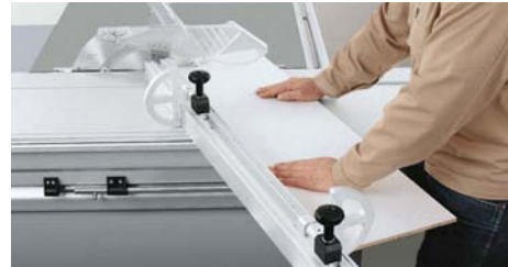
Mitre cut using one-sided mitre fence.
