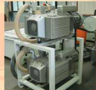
2x 10HP vacuum pumps are standard on the SELEXX/CHIEF. (Pump options available).
