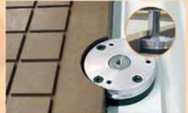
6 automatic steel pop-up pins on table for referencing sheet stock on models MATE, PAL and CHIEF. 12 steel pins on PRIMO.
