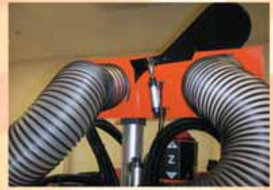
The SELEXX MATE, PAL, CHIEF and PRIMO provide for Automatic Dust Extraction Dampers on both Router Spindle and Drilling Head.
