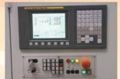
The standard controller on the ECO is the proven FANUC Oi Mate - MC.
