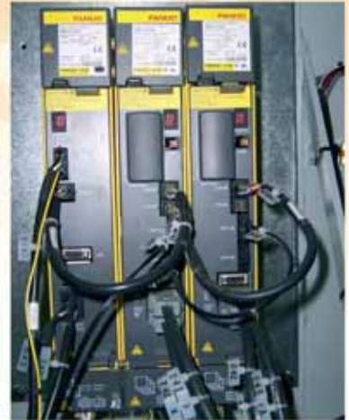
Models MATE, PAL, CHIEF and PRIMO are equipped with the FANUC Oi PC front end industrial controller. FANUC Servo Drive Motors on all axis.
