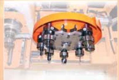
Each SELEXX model is equipped with an 8 position Automatic Toolchanger.
