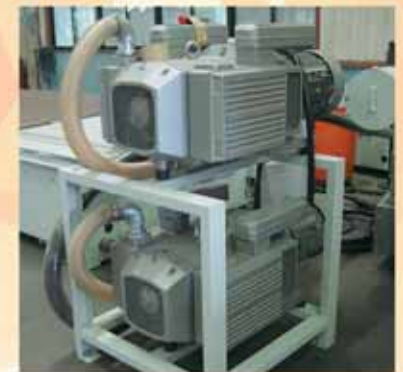
2x 10HP vacuum pumps are standard on the PRIMO. (Pump options available).
