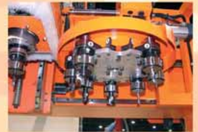
The SELEXX Series is equipped with HSK 63F Toolholder System on all models.
