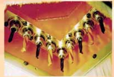
The 9 Spindle Vertical Drill is ideal for line hole drilling and individual point-to-point drilling for various applications. The Drill Head has Full Table Coverage.
