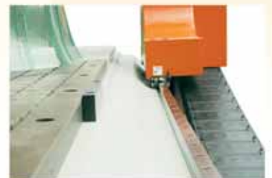
All SELEX models are equipped with precision linear guides on all axis.
