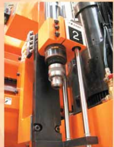
The ECO is equipped with a 0.25HP single spindle vertical drill head. Fixed rotation speed: 3.600 RPM
