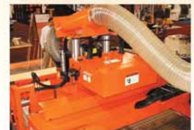
The SELEXX MATE, PAL, CHIEF and PRIMO provide for Automatic Dust Extraction Dampers on both Router Spindle and Drilling Head.
