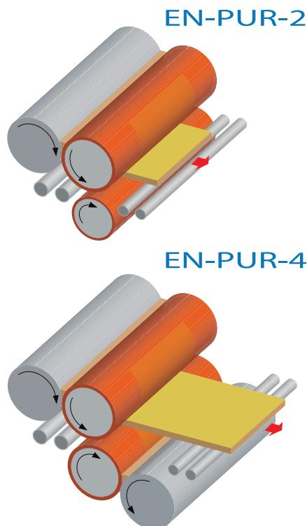
Gluing machine for the application of PUR hot melt glues on flat surfaces by means of a top/bottom spreader (EN-PUR-4), each one with a heat resistant elastomer coated application roller and an electrically warmed up metallic dosing roller.
