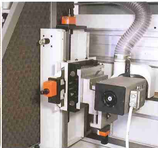
Universal milling unit with pneumatic jump, 0-90° rotatable.
