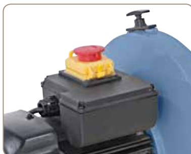
Lockable on and off switch in accordance with IP 54 standards and undervoltage release
