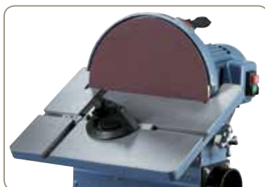
Tiltable grey cast-iron table features T-slots.
