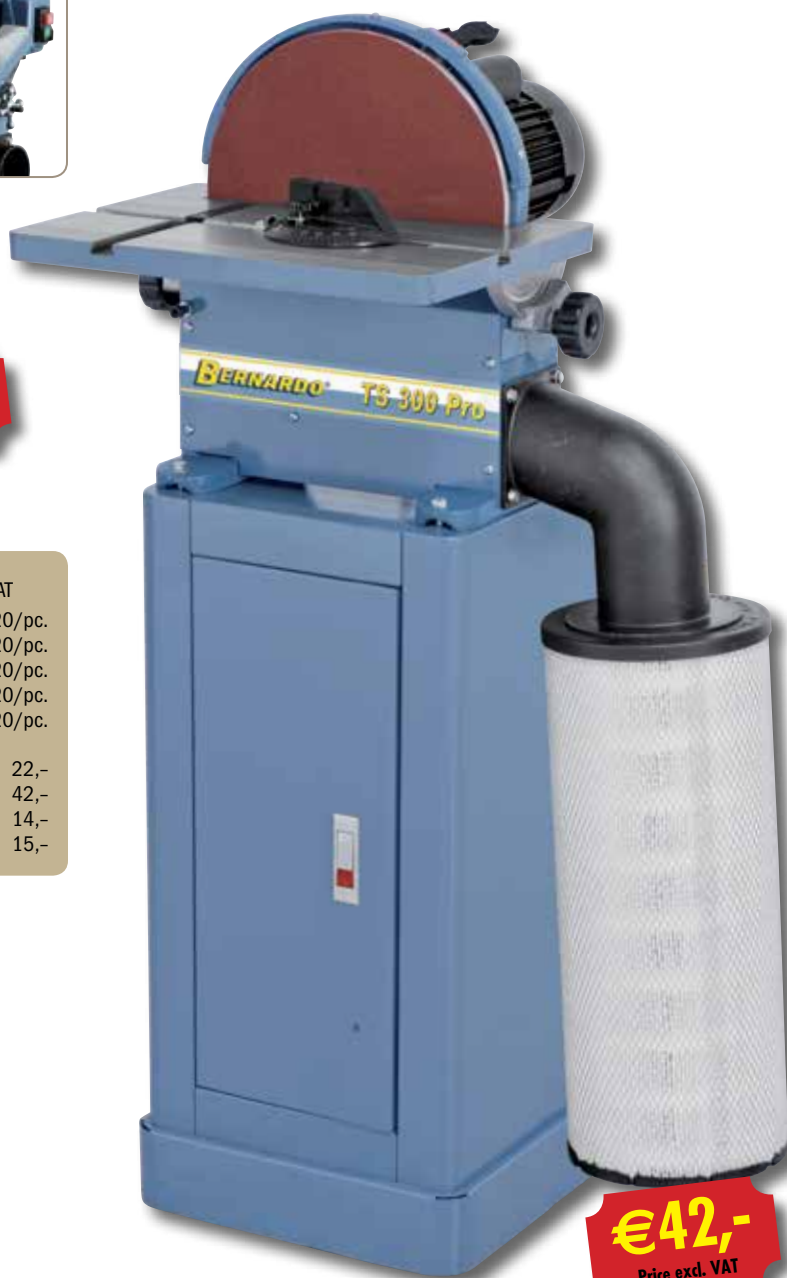
Tiltable grey cast-iron table features T-slots.
