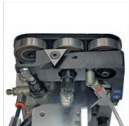
The Glue Scraper removes excess glue from the top and underside of the panel. This is the only model on the market fitted with 4 pneumatic cylinders for a top quality finish.
