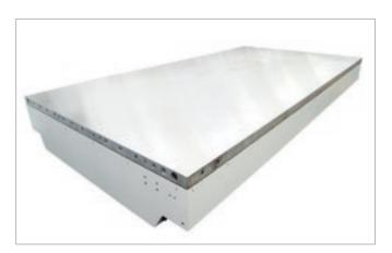
Solid steel platens, with holes for circulation of hot thermic oil guarantee perfect gluing. Platens are ground to ensure **perfect flatness and easy maintenance** to avoid glue spilling. Ground and polished pressing surface can be provided for special applications.
