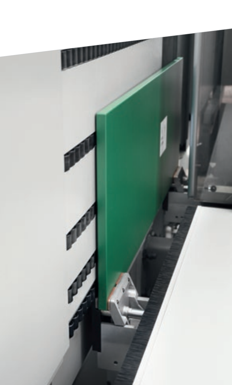
8-position tool magazine that manages different types of aggregates, thus increasing the machine's versatility.
