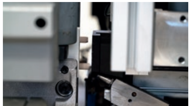
Unit for managing glue/dowel insertion with a patented system with tool change for recalling the work aggregate.
