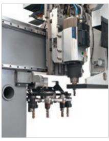
8-position tool change for each of the two electrospindles.
