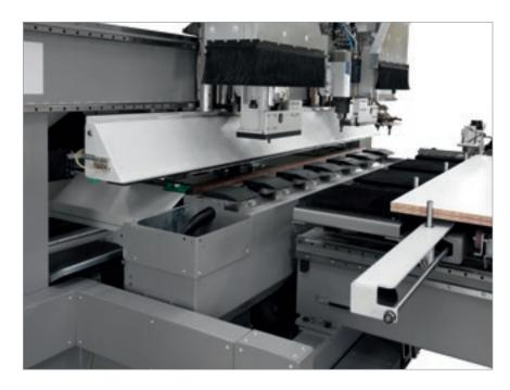
Nextstep allows users to machine two overlapping panels.
