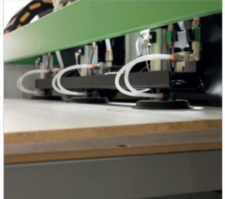
New suction cup loading system and dynamic vacuum.
