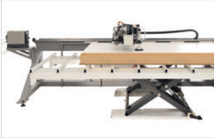
Loading system with scissor type loader.
