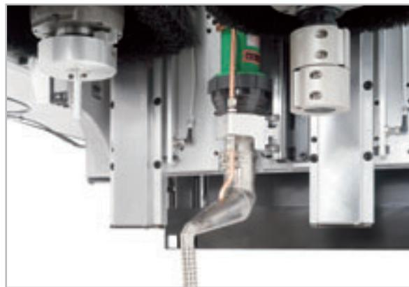
**Hot-air blower unit installed between the two electrospindles.**
