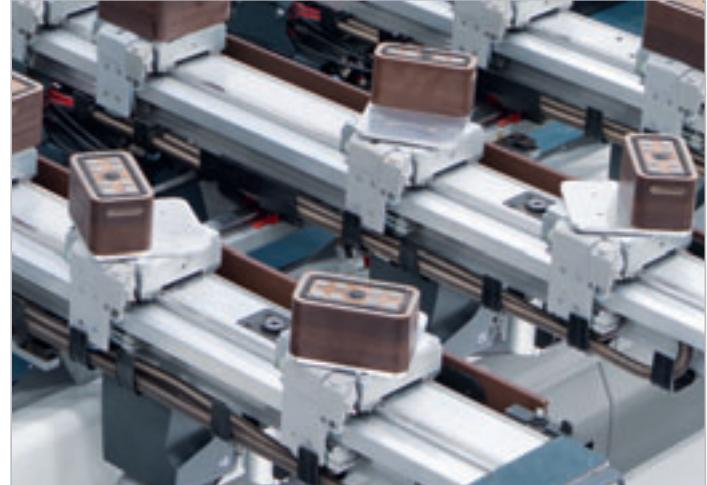
Vacuum cups with rubber to increase the locking of the pieces in presence of lateral forces.
