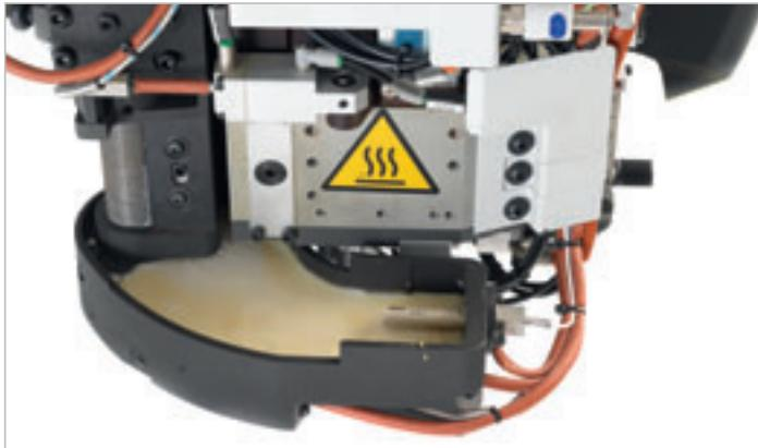
**Glue melted in the Teflon-coated glue pot with heating elements and sensor for the correct level control.**
