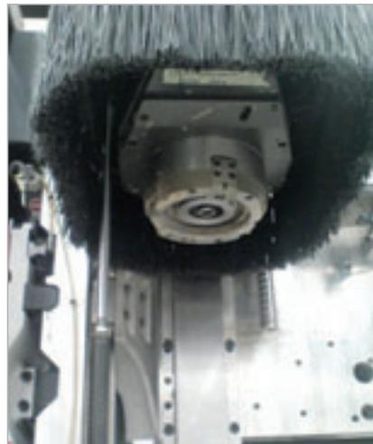
**Blower unit installed in the dust extraction system of the single electrospindle.**
