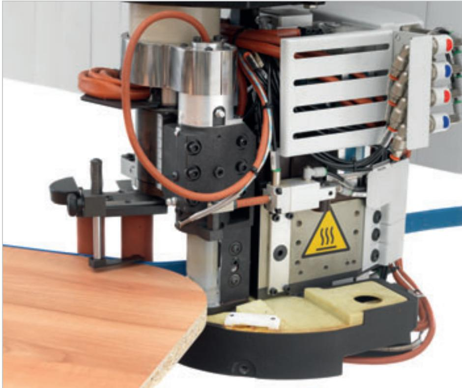
The glue is spread on the board in the same way as a linear machining, ensuring the same bonding quality. Able to use thin or transparent tapes (called 3D) using the same conditions of the thick and more resistant materials.
