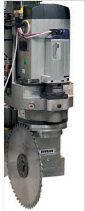
Multi-function units with electrospindle, C-axis and fixed aggregates.
