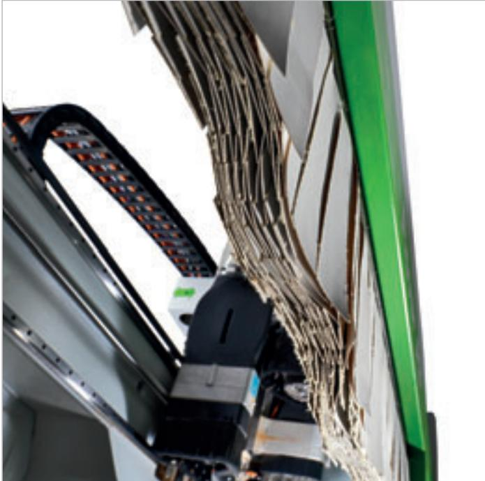
Pneumatically controlled mobile curtain guard system to enable piece loading operations and checking of the tool path during simulation.
