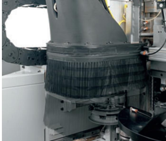
Suction hood adjustable to 5 positions (12 positions with 5-axes operating unit) from the NC.
