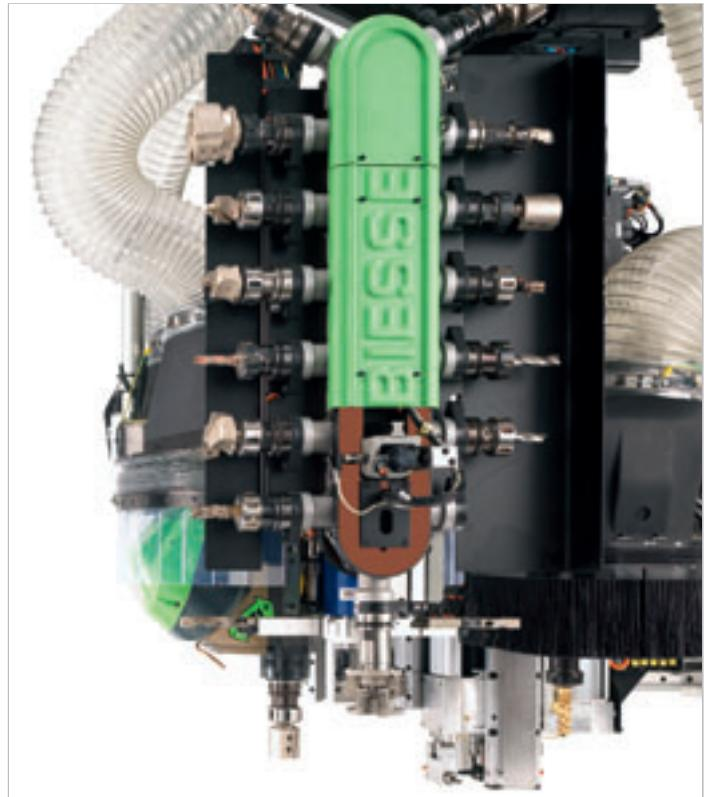
Belt tool changer with 15 places for 5 axes unit.
