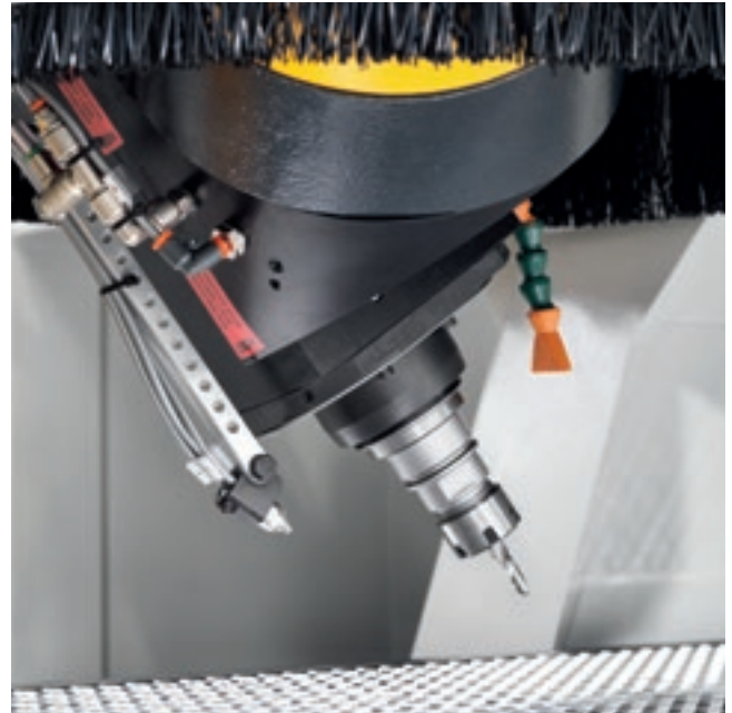
Electromandril 5 axes 13 kW 24.000 rpm.
