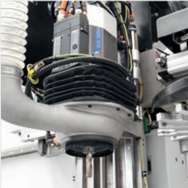
Electromandril 7,5 kW 36.000 rpm.
