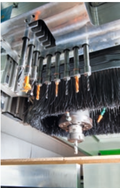
5.4 kW horizontal milling unit.
