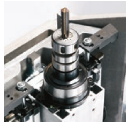
Electrospindles with HSK D-50 coupling.
