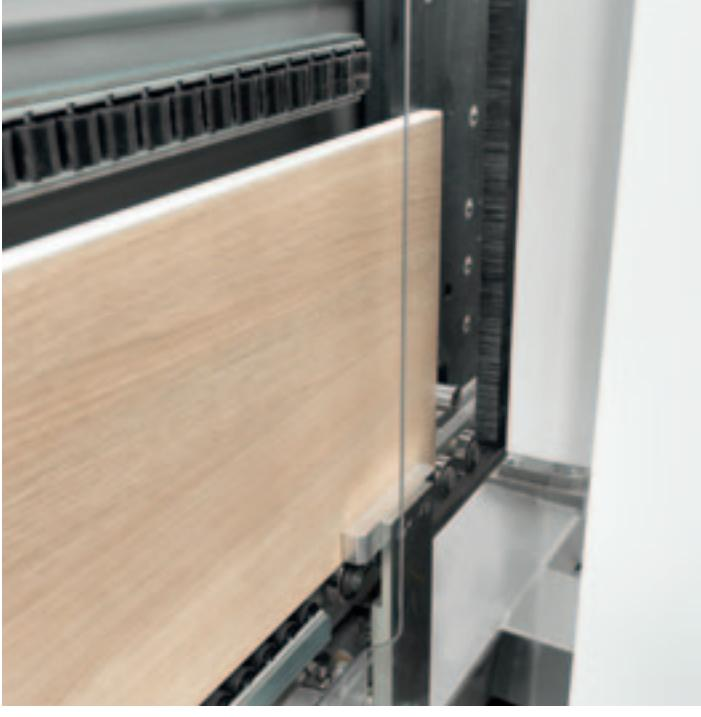
**Skipper V31** is the ideal solution for “just in time” production: set-up time = zero thanks to the panel handling by a fully automatic gripper.
