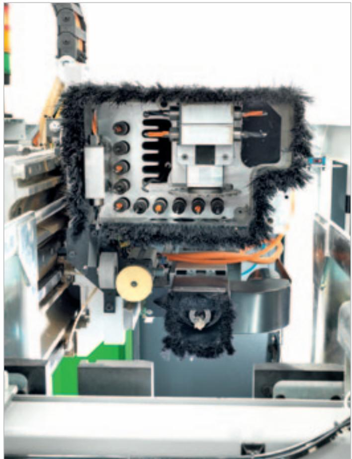
The operating unit configured with 10 vertical independent spindles + 6 horizontal spindles and 1 sawblade unit dia. 120 mm (optional electrospindle), complete all the machining on 5 sides of the panel.
