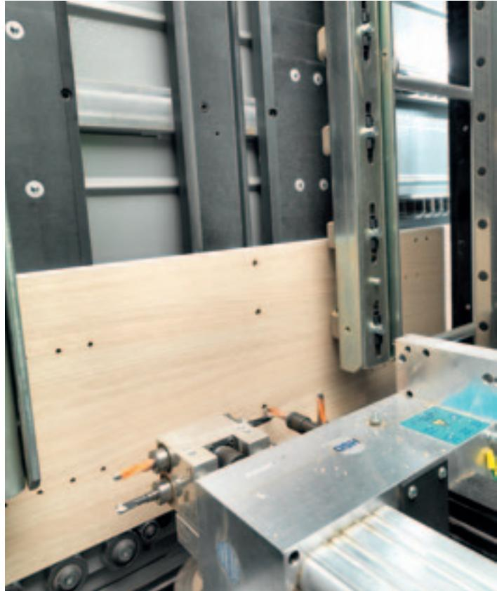
The presser rollers and the vertical pressure device provide maximum panel locking.
