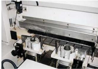
**Pre-Milling Unit** To rectify the edge of the panel with 2 HF motors - 12.000 rpm – 2.5 hp (1.8 kW) each and separate time entrance: 1st motor spinning anti-clockwise; 2nd motor spinning clockwise.
