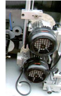
**Brushing Unit** To carry out the cleaning and polishing of the applied edge using cloth disc brushes with 2 motors 0.25 hp (0.18 kW) with cloth discs dia. 3.8" / 100 mm.
