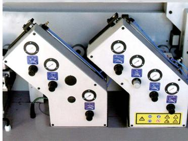
**End Trimming Unit** To carry out the trimming of edge excess at the front and rear portion of the panel with 2 tilting motors HF 0.5 hp (0.37 kW).
