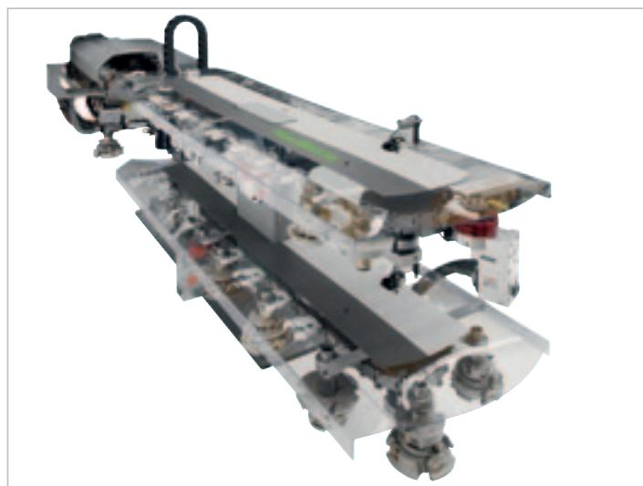
Flexstore C tool changer with 44 positions for the storage of tools of different types of windows and doors (optional).
