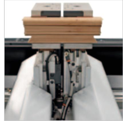
The special shape of the Finger locking modules allows also the machining of very short pieces.
