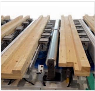
**Suction cups** with a vacuum fixing system making it easier to clamp even the thinnest panels.
