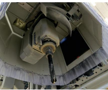
A wide range of machining operations can be carried out thanks to the **HSD electrospindle** (50-65 kW and 1000-15000 rpm) with its oil-lubricated bearings and HSK connection device. Equipped with a fixed deflector (automatically excluded when necessary).
