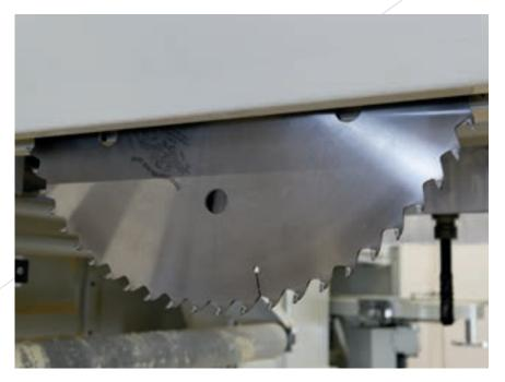
Maximum machining power, thanks to the **fixed blade** with its 1100mm diameter, that works at right angles to the table and can rotate 360°. Fitted with a special suction hood for cleaning both the piece and the machine.
