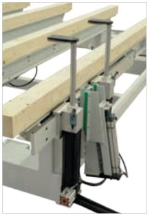
The **vertical clamps** are even able to block elements with a limited section, thereby increasing machining flexibility.
