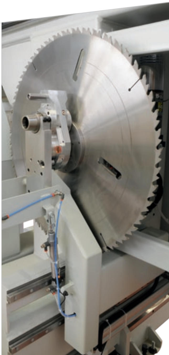
Blade magazine of 850mm diameter.
