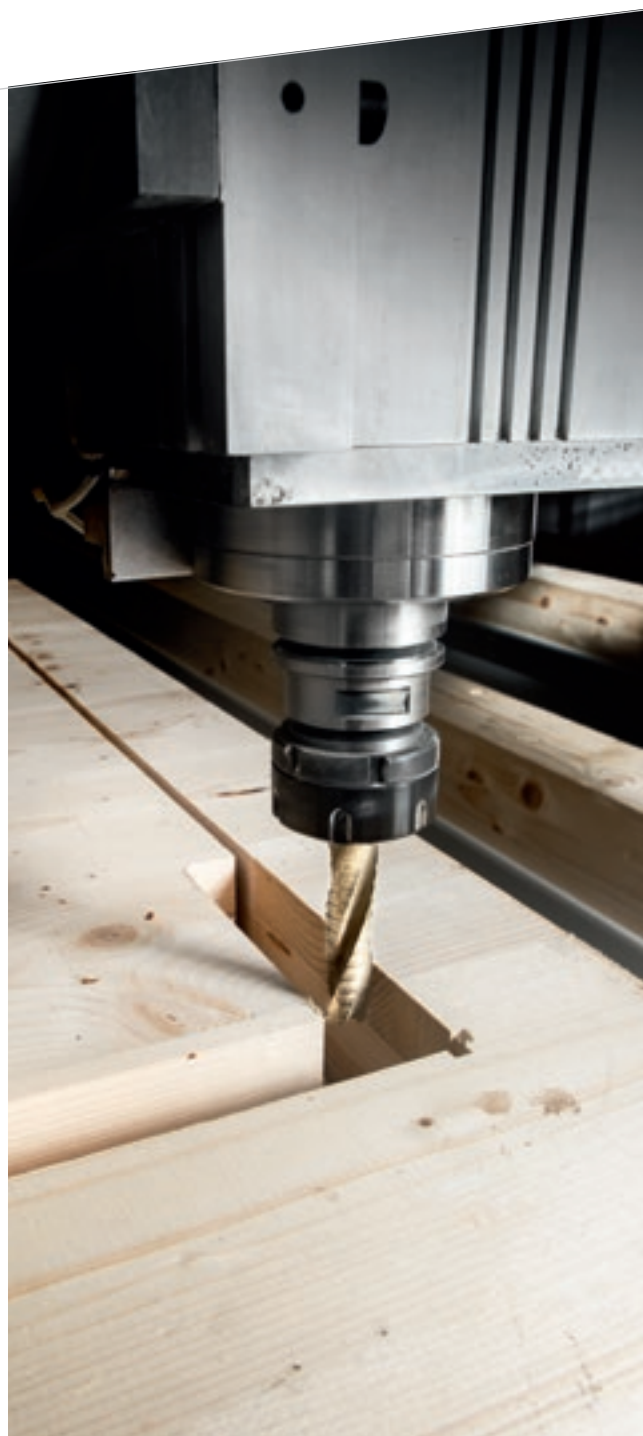
Top performance thanks to the 22kW synchronous electrospindle in the Y axis.
