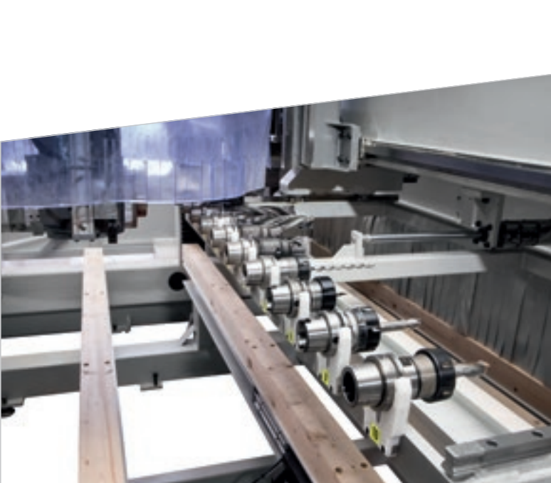
10-place tool magazine for quick tool changes.
