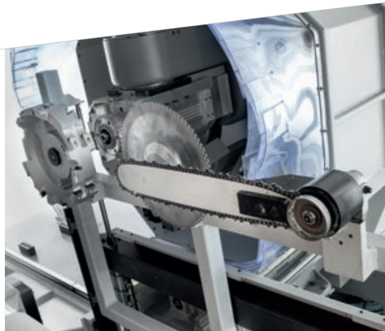
3-position magazine for large tools, including the chain tool if necessary.
