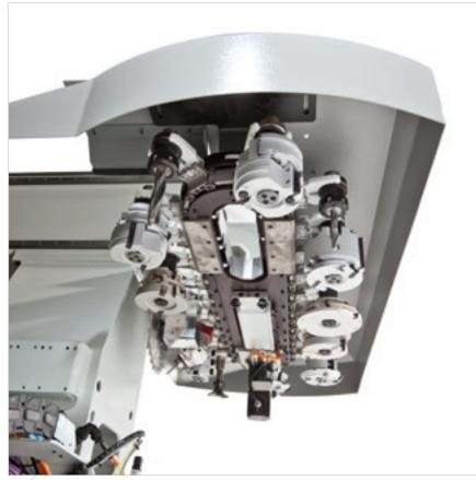
**Chain magazines** with 22 positions with distance between centres of 180 mm.
