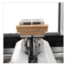
**Finger Clamps** always enable optimal clamping of the component. Even the shortest work piece is always secured using 2 clamps. It is possible to switch from one machining operation to the next with no need for manual intervention on the machine.
