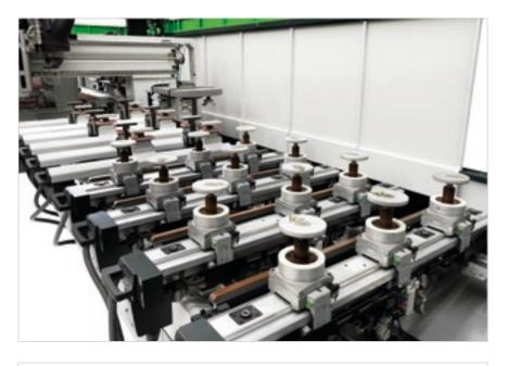
Dedicated **EPS table** for arches, squaring and special machining operations, to be equipped with Hyperclamps or vacuum modules.
