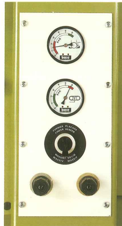
Control panel pneumatics
