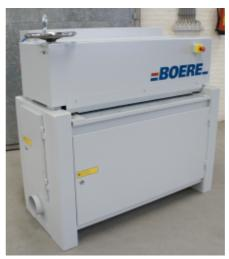
The brush machine has been especially developed for cleaning of carpet tiles, car mats, etc., and is therefore very apt for hire companies. The special construction of the fibre brush provides for brushing the tiles in the right hair direction so that the tiles look as new when they come out of the machine.
