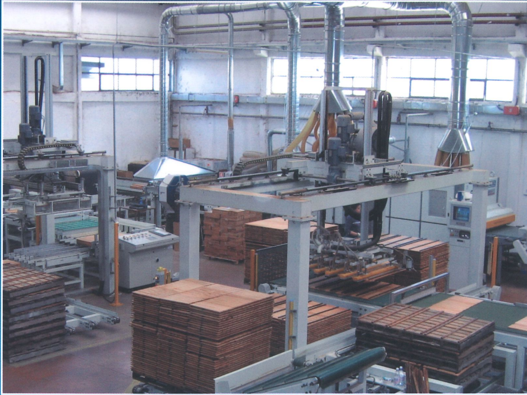
17 - Loading and unloading for sanding line.
