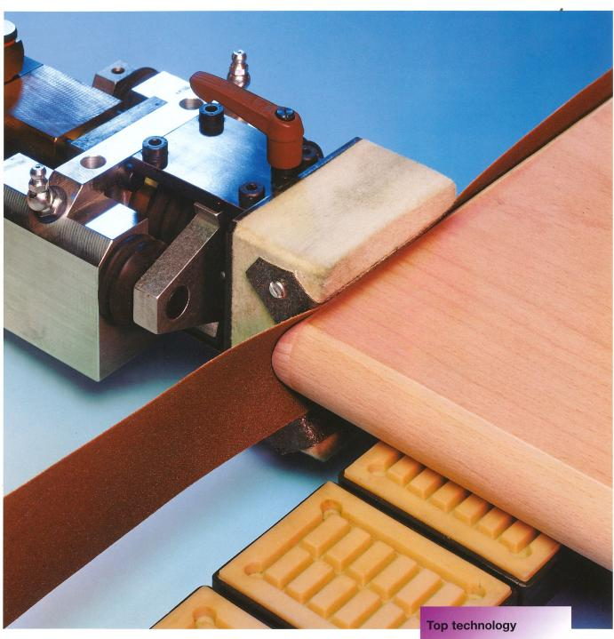
Profile trimming and sanding machine Optimat SP
