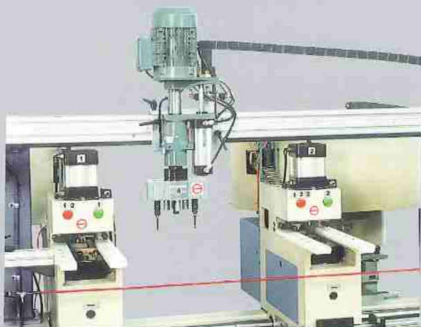
TMB-3001 WITH VERTICAL DRILL WITH ELECTRICAL MOTOR
