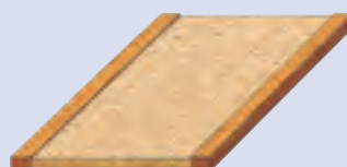
Chipboard with solid wood edge banding
