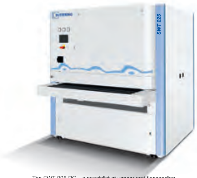
The SWT 225 RC – a specialist at veneer and finesanding.
