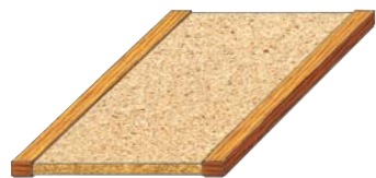
Chipboard with solid wood edge band
