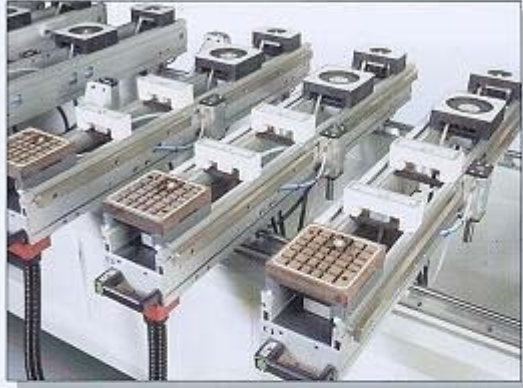
Vacuum cup clamping system, differing according to the size of the pieces.
