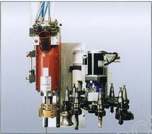
Head mounted rotary tool changer system: 10 positions
