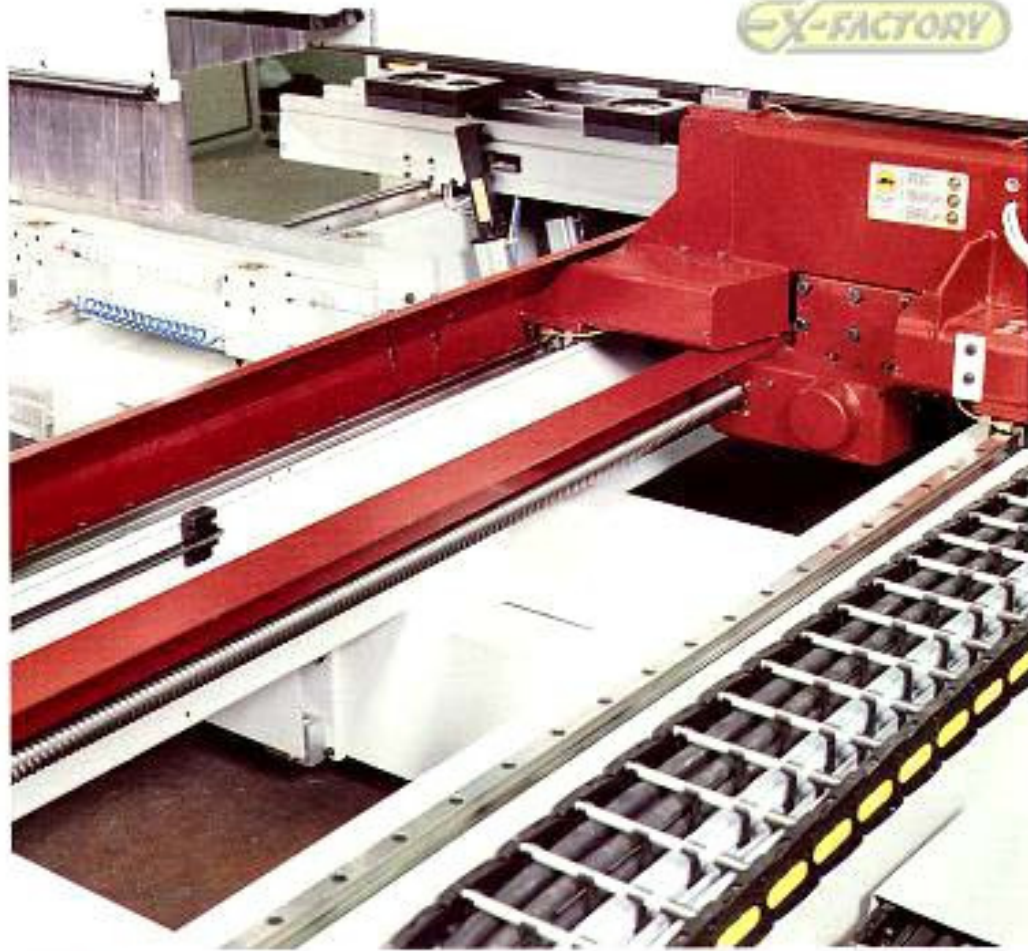
Square rails on the "X" axis, circulating ball nut and lead screw.
