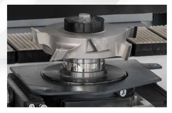
• DIA tooling for the roughing process prior to the outlining
